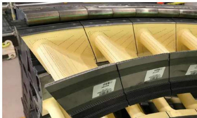
GT13E2 MXL VANES AND STATOR HEAT SHIELDS INSTALLED IN TVC
