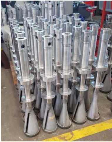
GT13E2 EV BURNER / AEV BURNER and LANCES NEW MANUFACTURING / FLOW TEST AND PACKAGING
