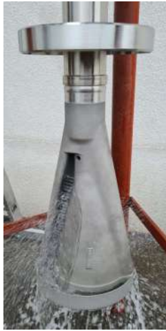
GT13E2 EV BURNER / AEV BURNER and LANCES NEW MANUFACTURING / FLOW TEST AND PACKAGING
