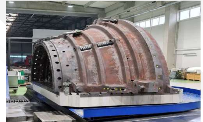
GT13E2 TURBINE VANE CARRIER REPAIR
