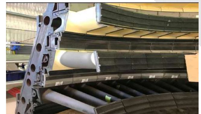
GT13E2 MXL VANES AND STATOR HEAT SHIELDS INSTALLED IN TVC
