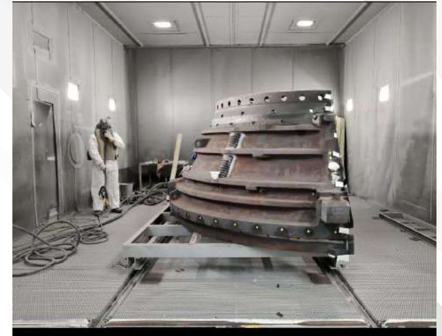
GT13E2 TURBINE VANE CARRIER
