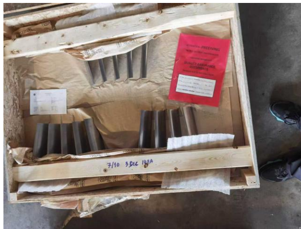
Photo 6/8 — Item 1: 3rd Stage Bucket 9FA (P/N 100T088G011), wooden box packing
