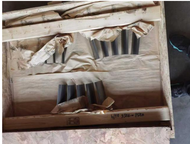
Photo 7/8 — Item 1: 3rd Stage Bucket 9FA (P/N 100T088G011), wooden box packing
