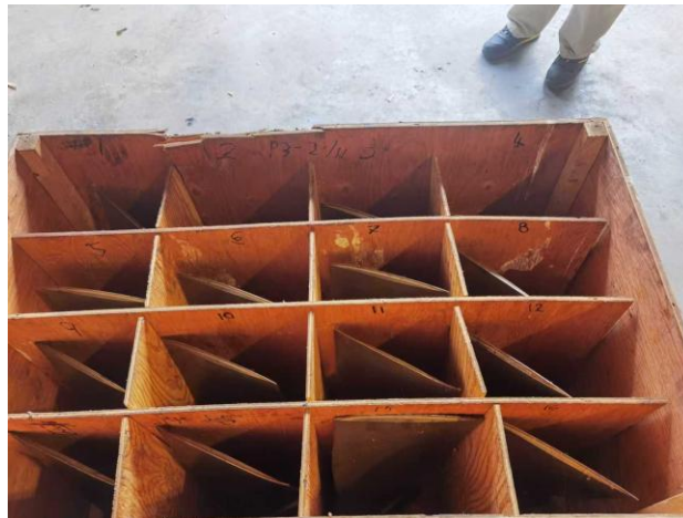
Photo 8/8 — Item 1: 3rd Stage Bucket 9FA (P/N 100T088G011), wooden box packing
