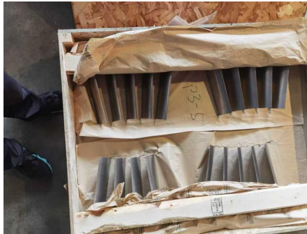
Photo 5/8 — Item 1: 3rd Stage Bucket 9FA (P/N 100T088G011), wooden box packing
